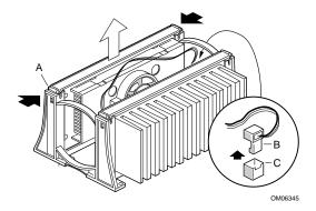
Figure 5. Removing a Processor
