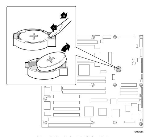
Figure 9. Replacing the Lithium Battery
