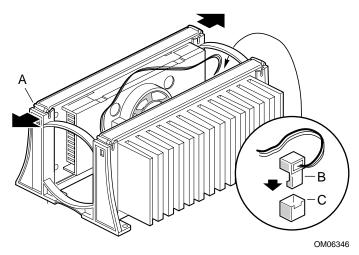
Figure 8. Locking in the Processor
