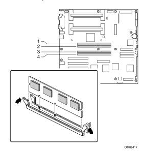
Figure 4. Installing DIMMs
