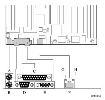
**Figure 1. Back Panel Connectors**
