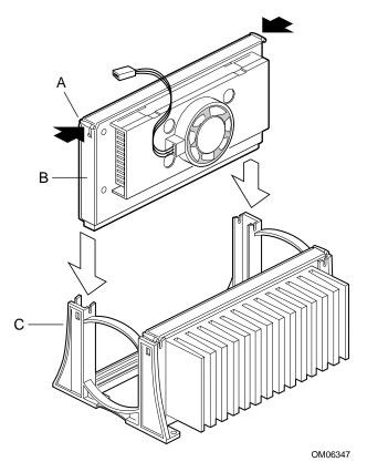
Figure 6. Installing a Second Processor
