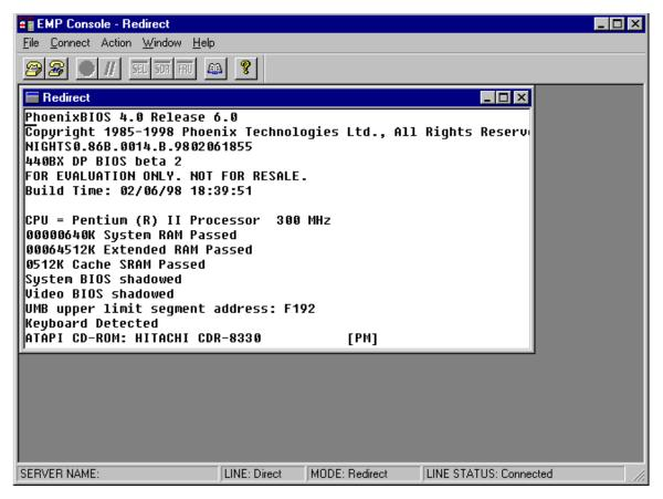
Figure 12. EMP Console in Redirect State
