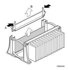
Figure 7. Removing a Termination Board
