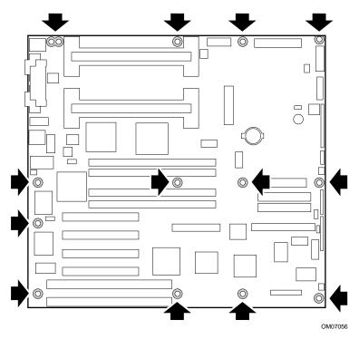
Figure 3. Server Board Screw Hole Locations
